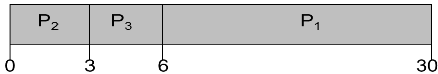
Figure 2.9. Sample arrangement of process in SJF scheduling
